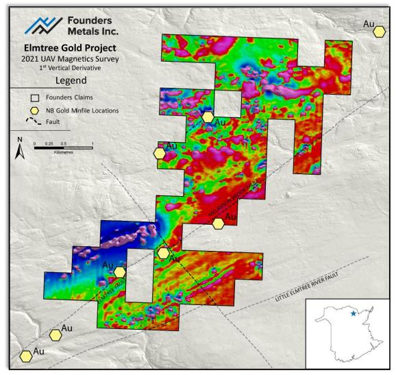
Figure 1 – Map of 2021 UAV/drone magnetics survey ( $1^{st}$  vertical derivative shown). Significant regional structures were added to demonstrate the spatial link between gold mineralization and northeast-trending structures.
